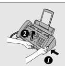
2 Remove the used film and empty spool.
